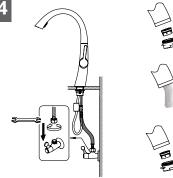
Attach the water lines to your main water supply lines. Ensure that you are connecting the hot and cold lines appropriately. Remove the aerator. Run water and check for leaks. Reinstall the aerator
