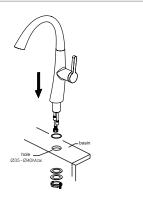
Make sure there is a 35mm-40mm hole on the basin before installing the faucet, Unscrew the fitting ASSY from the bottom of the body, then pass the body through the hole, don't forget to fix the o-ring between the bottom of the faucet and the basin.
