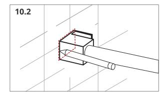
Remove the stoppers brackets from the running rail  $% \left( 1\right) =\left( 1\right) \left( 1\right) \left($
