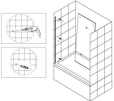
**04** Apply silicone inside the wall profile as shown
