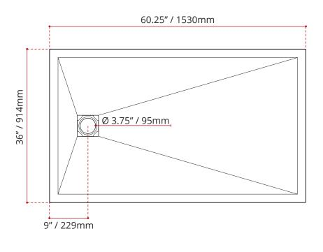
DISCLAIMER: Measurements may vary  $\frac{1}{2}\, 1\!\!\! \mbox{\ensuremath{\mbox{\sc d}}}{}^{*}$  (Diagram Not to scale)
